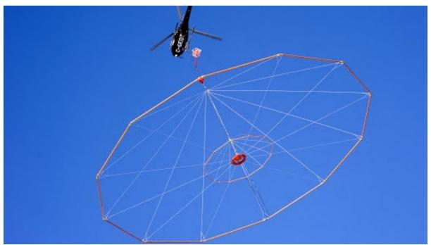
Figure 1: VTEM MAX<sup>™</sup> system in flight at Halls Creek Project (Photo – Geotech)
