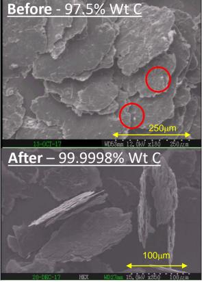
Impurities (circled-top) tend to occur on top of the flakes not embedded into the flake layers making for "easier" purification;
