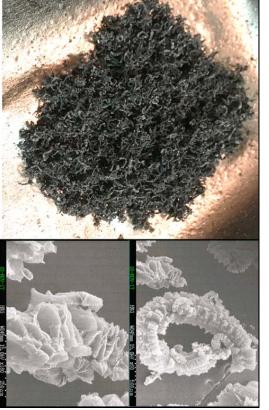
Expanded graphite "worms" produced from +60 mesh fraction of HXGCON 1 precursor flake: optical (top), SEM (bottom).
