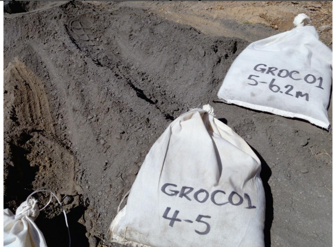
Figure 1B Auger hole showing the flake graphite – rich intercept.
