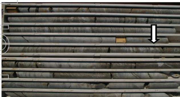
Figure 2A: Trays 1 and 2 from drill hole T2GDD003 showing graphite intercepts from the interval 101.6 m to 110.55 m.
