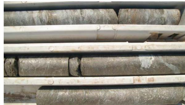
Figure 2B: Detail of the high grade flake graphite intercept arrowed in Figure 1A.
