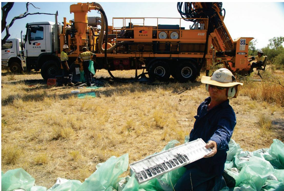
Figure 2: Displaying drill hole chips from a graphite intercept in an RC drill hole and detailed below.
