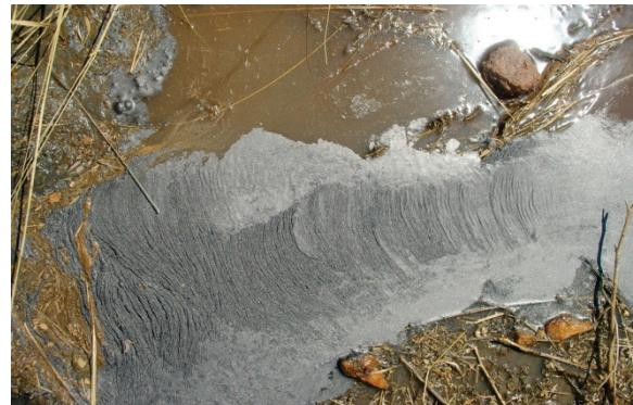
Figure 5 Flake graphite accumulating on drill water
