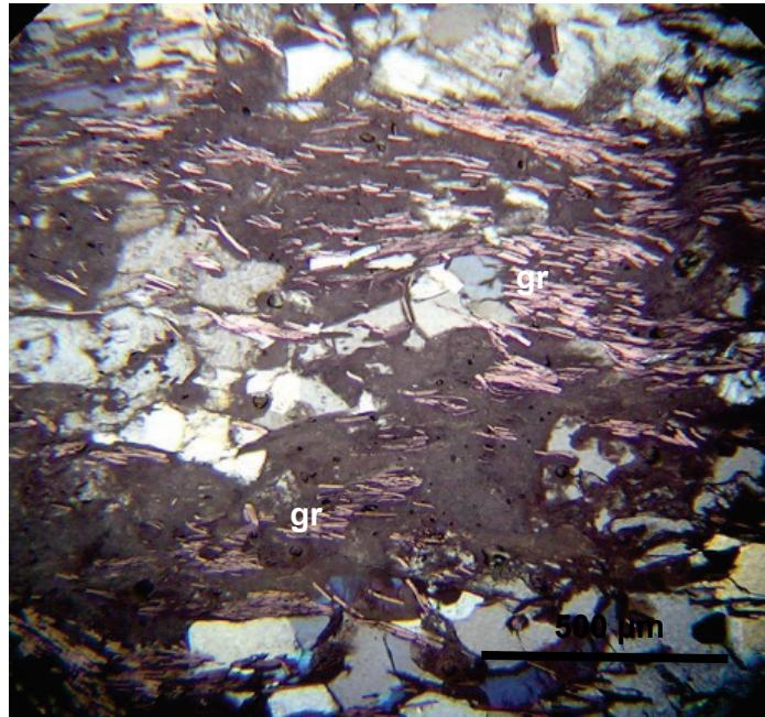
Figure 6 Photomicrograph of flake graphite (gr) at Target 2. Width of photograph 1.5 mm (or 1500  $\mu$ m).
