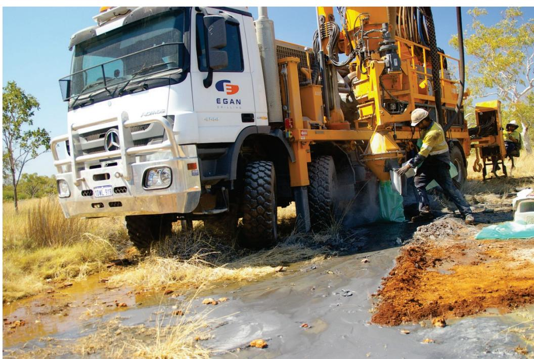
Figure 3: Flake graphite producing a distinctive sheen on drill water from a RC drill hole at Target 2
