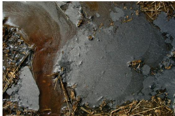
Figure 4 Flake graphite sheen on drill water
