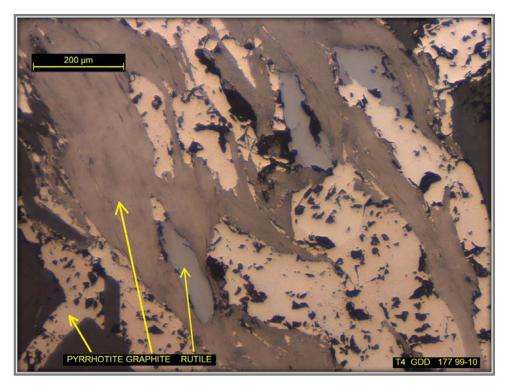
Figure 1: Photograph of T4GDD177 (54.72 - 58.02m) showing strong flake graphite mineralisation
