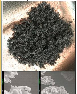
Expanded graphite "worms" produced from +60 mesh fraction of HXGCON 1 precursor flake: optical (top), SEM (bottom).
