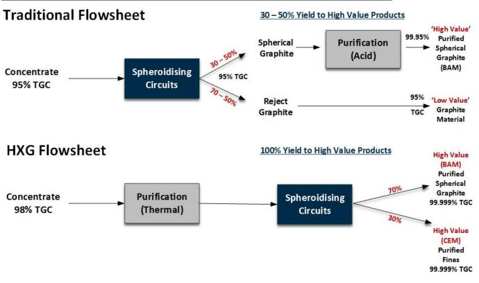
HXG is proposing an innovative downstream flow sheet based on:
