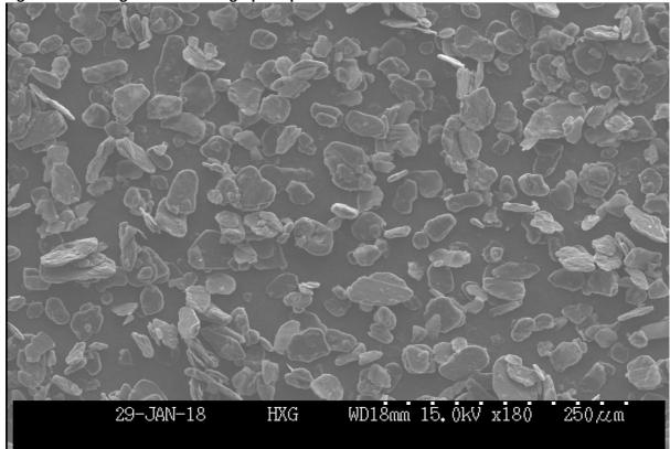
Figure 4. Scanning Electron Micrograph of purified McIntosh flake at <140 mesh size fraction.
