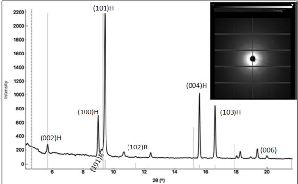
Figure 2: APS XRD Scatter Plot for McIntosh purified flake.
