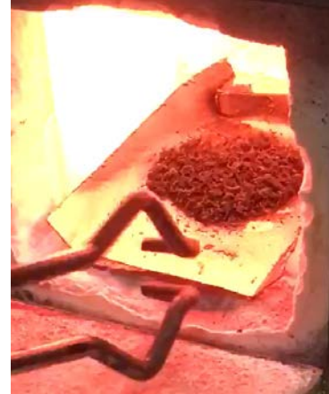
McIntosh flake graphite expanding with exposure to heat
