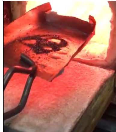
McIntosh flake graphite expanding with exposure to heat
