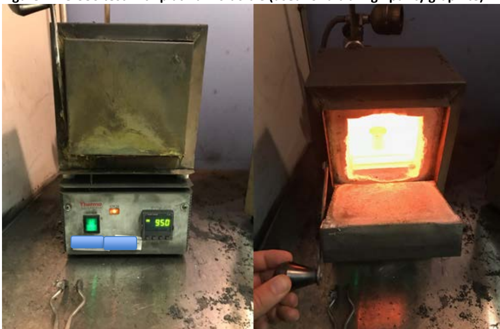
Figure 2. LOI950 test with platinum crucible (used for ultra-high purity graphite)
