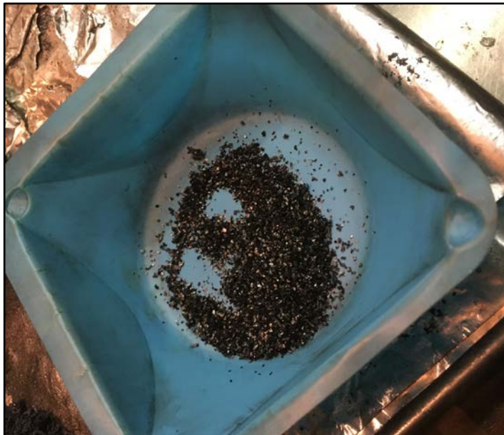
Figure 4. Dry acid intercalated +60 Mesh McIntosh graphite prior to heat expansion.
