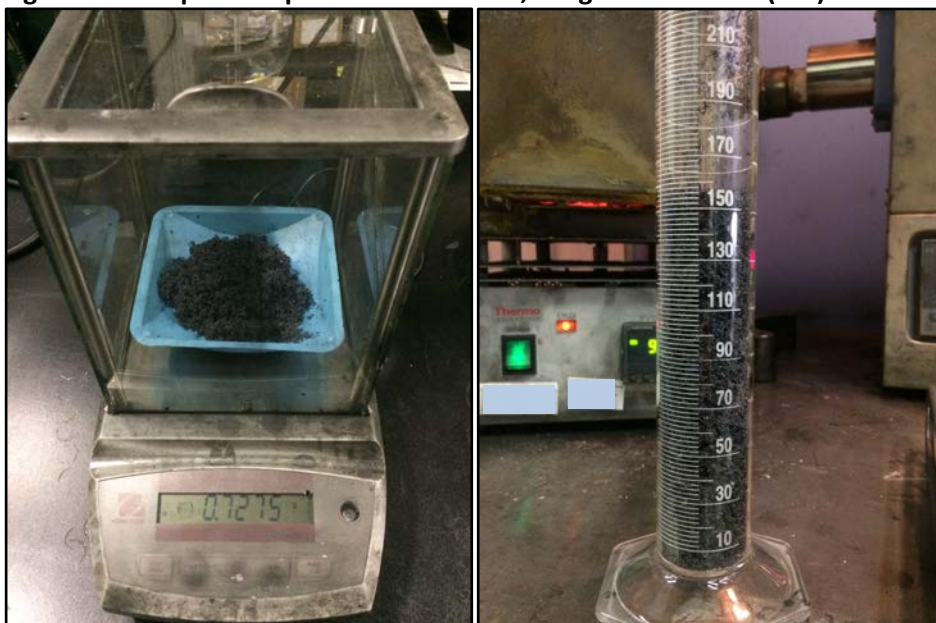
Figure 1: Example of expansion calculation; weight of material (left) and volume (right)
