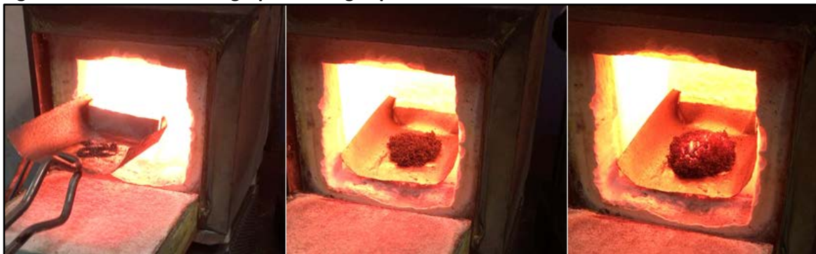
Figure 5: Acid intercalated graphite being expanded in a furnace at 950°C.
