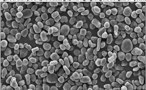
Figure 1: Example of spheroidised graphite highlighting the elongate or "potato" shapes.
